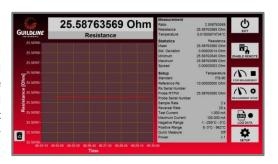
All 664oT Bridges provide a full 10.5 digits of resolution and the ability to **graphical see** the data (trending). You can have the data presented in a **summary or detailed format** right on the Bridge Screen or available via PC based BridgeWorks Software. The 664oT Temperature Bridge provides the **Measurement and Uncertainty Analysis** you need as a Metrologist or to meet the requirements of ISO 17025 Accreditation!
