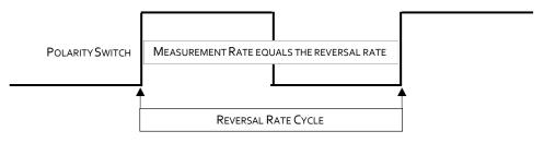
reversal rates are typically 20 seconds or more. This equates to a reading every 20 seconds.
