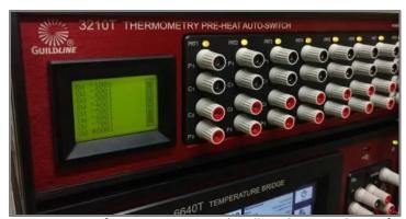
initiated while the Bridge is unattended. All user definable test variables, such as excitation current, pre-heat current, measurement speed, reversal rate etc can be programmed on a per test basis, giving the users full control and flexibility in conducting well designed measurements, and for calibrating temperature probes.
