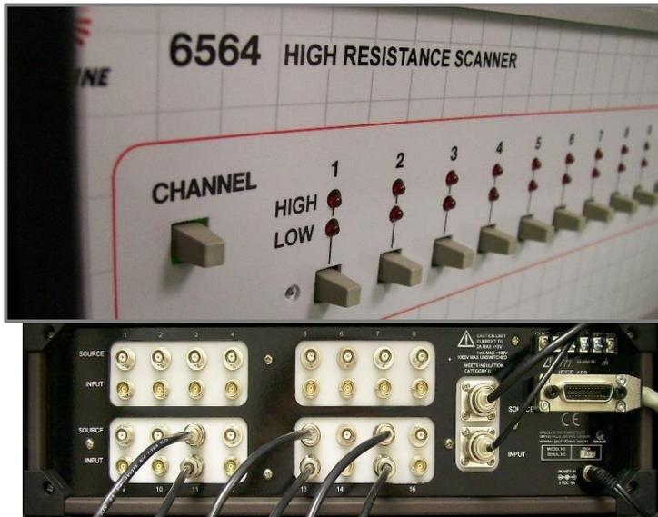
Guildline's 6564 High to Ultra-High Resistance Scanners are the first commercial scanners capable of operating with measurement capabilities to  $10 \text{ P}\Omega$ 's and at voltages to 1000 Vdc. This capability greatly improves the measurement and calibration throughput of high and ultra-high ohm resistance measurements. Standard laboratories can easily and quickly automate measuring single or multiple resistance values.
