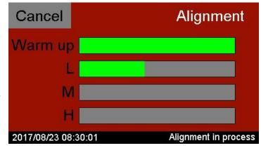
All operations are performed via a front panel touch screen or can be automated via a computer connected by Ethernet/IEEE or USB. Manual configuration and control of the divider output is performed by simply pressing the appropriate screen entry. Both the touch screen and Ethernet/GPIB/USB interfaces are controlled by a microprocessor which is kept isolated from the temperature controlled analogue circuits that are part of the voltage divider network and
