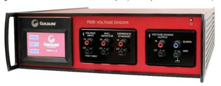
Special care has been taken to minimize thermal offsets and noise during use, and during the 7520 self-alignment/self-calibration. The voltage reference, resistive voltage divider networks, and optical null detector are all inside a thermally
