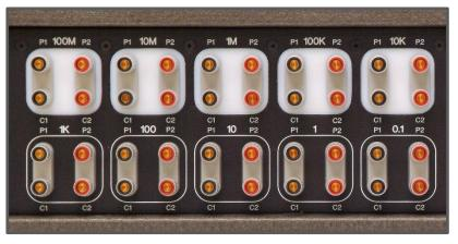
**Low Ohms Model** - Given the performance of the Model 6634A standard values from 0.1  $\Omega$  to 100 M $\Omega$ , customers have requested that Guildline provide a 6634A with low value resistance standards - so we obliged. We now have a **Low Ohms model** that has 3 elements from **0.001**  $\Omega$  to **0.1**  $\Omega$ . You can also have any special value (e.g. 5 m $\Omega$ ), but the unit is limited to 3 elements due to the larger size of the low value elements.
