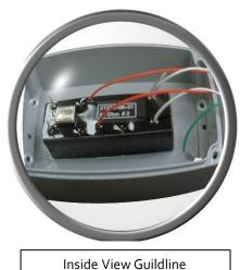
left is an individual Guildline Resistance Standard. Note that in this design you can see the spacing between the C1 and C2 Terminals showing that multiple elements are used in the MAIN element build up. In fact, the primary (1<sup>st</sup>) trim resistor used in this Guildline Resistance Standard is
