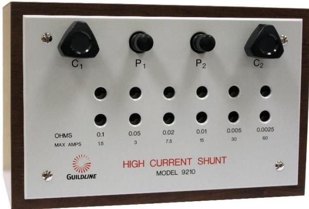
**Guildline Model 9200 and 9210** are compact four-terminal Multi-Value Resistance Standards. These standards are in a durable Formica case, with all terminals and adjustments available at a panel on the top surface. Separate current and potential terminals are provided. Two range plugs, inserted as a pair in the top panel, select one of several decade resistance values. Both models produce a maximum DVM reading up to 0.15 volts.
