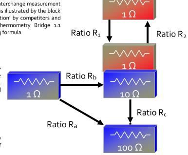
This **Multi-Ratio** capability allows users to extend the calibration interval of the Thermometry Bridge while still maintaining a high level of confidence, thus saving thousands of dollars each year in support of the instrument. With an annual verification, a Guildline 6622T Thermometry Bridge typically can go five years between calibrations.
