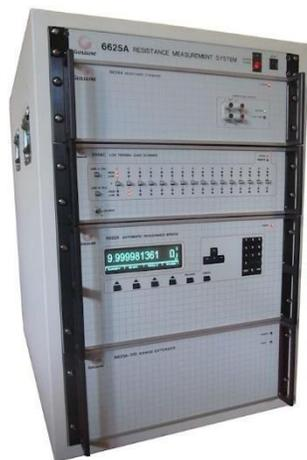
The **6625A Measurement System** is highly configurable to meet wide ranging workload requirements. The 6625A is capable of resistance measurements using **6634A models** from  $1 \mu\Omega$  up to  $1 \text{ G}\Omega$  at 1000 V with a single 6622A DCC Bridge.
