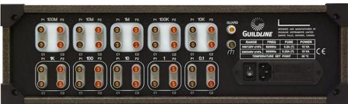
For the Normal Ohms Configurations, there are 10 standard resistance values available covering the range of 0.1  $\Omega$  to 100 M $\Omega$ . Each resistance element is isolated and has 4-terminal connections on the rear panel. The resistance elements are maintained at approximately 30  $^{\circ}\text{C}$  in a temperature stabilized chamber. Each element is built with Guildline's "true" multi-element design.
