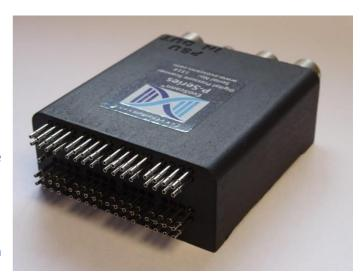
EvoScann® P64-D is a miniaturised pressure scanner designed specifically to meet the stringent demands of the aerodynamic testing industry where development is rapid and continuous. Utilising the latest in miniature scanner technology, P64-D is at the forefront of pressure measurement in challenging aerodynamic locations. The P64-D has been designed, from the start, with physical size, weight, accuracy and functionality in-mind.
