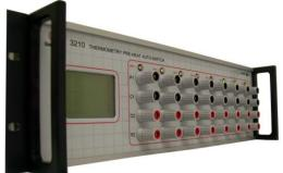
**New Thermometry Adapter**: The new Guildline 3210 Thermometry Adaptor, and optionally a Low Thermal Matrix Scanner, is included with the System. Every one of the eight channels on the model 3210 Thermometry Adaptor has its own pre-warm capability and automation support. The channels in pre-warm are identified with a yellow LED indicator while the selected channel being measured has an active Green LED indication.
