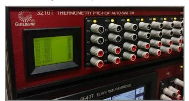
initiated while the Bridge is unattended. All user definable test variables, such as excitation current, pre-heat current, measurement speed, reversal rate etc can be programmed on a per test basis, giving the users full control and flexibility in conducting well designed measurements, and for calibrating temperature probes.
