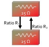
The 1:1 measurement ratio can be easily calibrated and verified by interchange measurement tests using two stable standard resistors of same nominal values, as illustrated by the block diagram to the right. Bridge 1:1 measurement ratio error  $e_i$  (in ppm) is calculated using the following formula:
