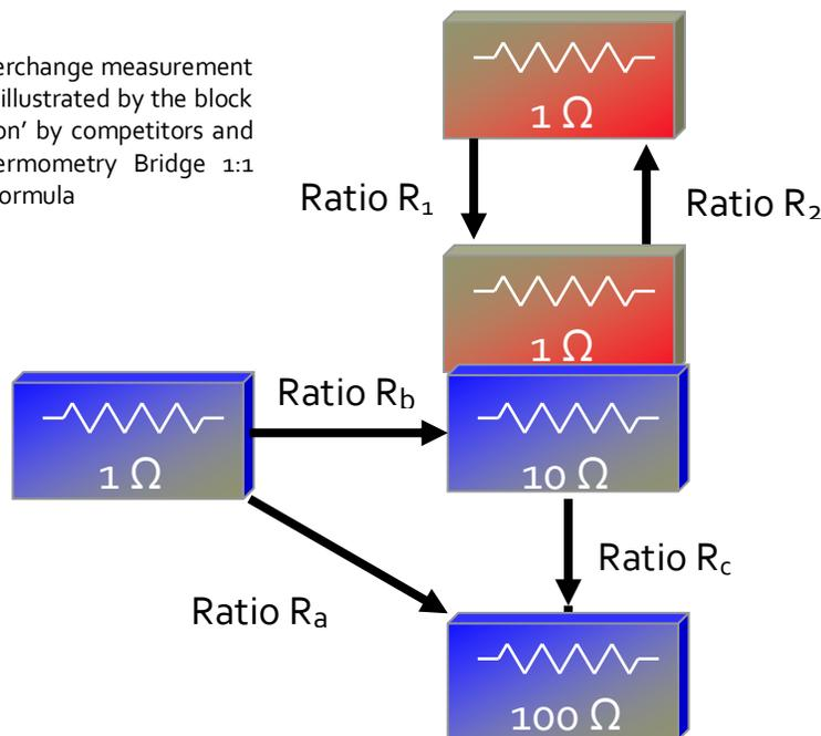
This **Multi-Ratio capability allows users to extend** the calibration interval of the Thermometry Bridge while still maintaining a high level of confidence, thus **saving thousands of dollars each year in support** of the instrument. With an annual verification, a Guildline 6622T Thermometry Bridge typically can go five years between calibrations.
