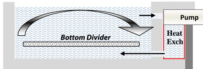
The discharge from the heater exchange is directed under the bottom divider of the tank. A much larger volume of liquid gets drawn down under the false bottom through a slot at one end. This flow mixes with the heat exchanger discharge. As it emerges from under the bottom divider, the liquid is so close to the mean tank temperature, that **gradients are less than 0.002 °C** throughout the bath.
