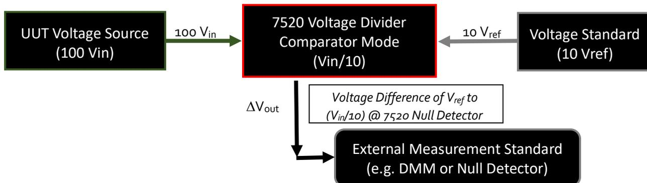
In addition, when operated in the Comparator mode of operation, the polarity of the Voltage Reference can be switched inside the 7520 manually or automatically. This enables fully automated polarity switching, and thus a fully automated calibration because the wires connecting the Voltage reference do NOT have to be manually switched to change the polarity. This also speeds up the calibration process because there is no wait time required due to switching the Voltage reference leads.
