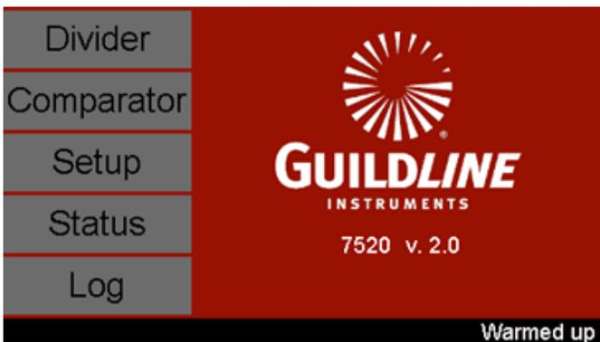
You can choose to use the 7520 as a “Divider” taking the voltage from an input reference and generating an output voltage based on 1:1, 1:10, 1:100 and 1:1000 ratios. This mode is typically used to calibrate a working voltage reference or the
