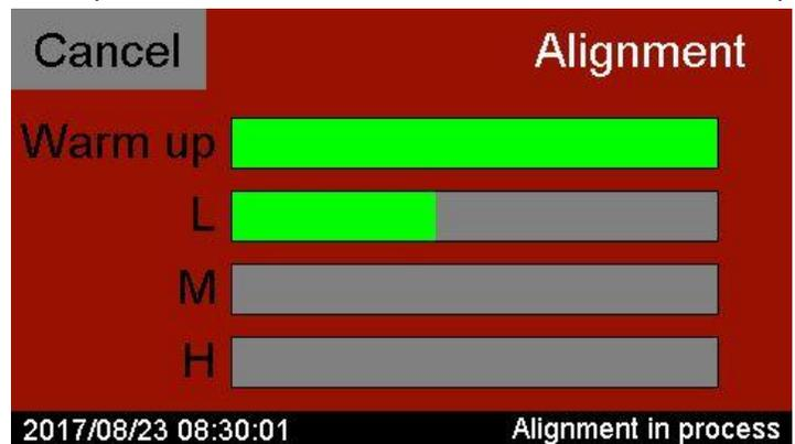
All operations are performed via a front panel touch screen or can be automated via a computer connected by Ethernet/IEEE or USB. Manual configuration and control of the divider output is performed by simply pressing the appropriate screen entry. Both the touch screen and Ethernet/GPIB/USB interfaces are controlled by a microprocessor which is kept isolated from the temperature controlled analogue circuits that are part of the voltage divider network and
