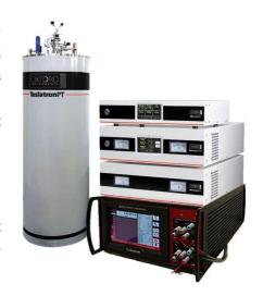
while taking a measurement. Competitors require that the measurement be stopped, parameters reset, and the measurement restarted. As a result measurement data is lost. Additionally, internal utilities reside within the BridgeWorks software to enhance and **simplify the calibration of the 664oQ** QHR Bridge by using the Guildline 6634A Series of Temperature Stabilized Resistance Standards.
