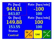
Ethernet. All the important air data functions are simultaneously displayed on all interfaces, constant screen or menu changes are not required. Readings of both commanded and measured test values are displayed.
