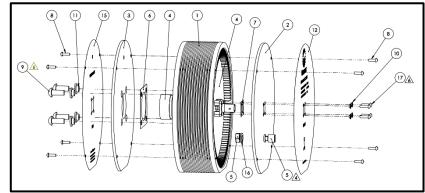
It starts with a well designed, EMI shielded, ruggedized case. You can see from the exploded diagram that the 7340/7350 case protects the resistive elements and all shunt circuitry. The shielded case also greatly reduces EMI effects. This design ensures there are no long electrical paths or traces which reduces phase shifts. All these features mean you do not have to worry about compensating for AC measurement parasites during the measurement or using special laboratory conditions.
