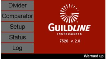
self-alignment circuitry. This high isolation ensures no offsets will be present in measurements due to leakage or noise from the rest of the circuitry inside the 7520. An easy to use Operating Menu is provided as per the screen image to the left. An operator has five selections from the Main Menu.
