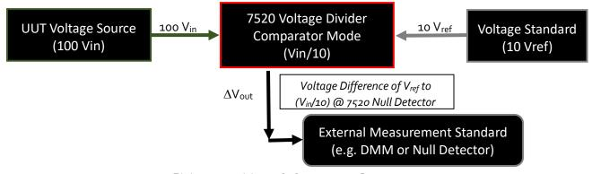
In addition, when operated in the Comparator mode of operation, the polarity of the Voltage Reference can be switched inside the 7520 manually or automatically. This enables fully automated polarity switching, and thus a fully automated calibration because the wires connecting the Voltage reference do NOT have to be manually switched to change the polarity. This also speeds up the calibration process because there is no wait time required due to switching the Voltage reference leads.
