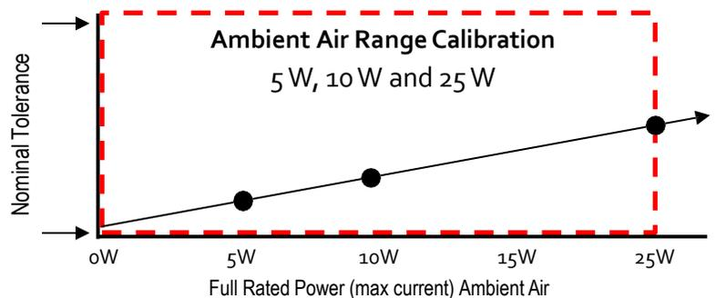
**Cooled (92310 Option or Oil)** - when the shunt is used with the 92310 option (forced air convection), the shunt can be used up to a maximum nominal power dissipation level of 100 watts and will vary for specific shunt values from 90 W up to 125 W. The calibration points are nominal 10 W, 25 W and the specified full scale current for cooled operation. Additional or optional points can be specified for a nominal fee.
