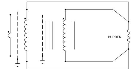
Typical Transformer Connections
