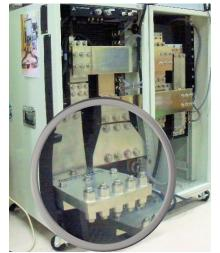
How good is the 6623A-PCS? Measurement results from a 1000 Ampere IntercomparisonoftwoNMIs(TestResultsshownbelowright)camewithin5ppmofeach other. One setup was a Guildline 6623A-PCS/4000A System with our 66259 Controller. This system is shown to the left.
